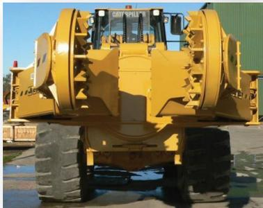
The **JEC Dual-Arm Tyre Handler** range has been engineered to provide cost effective tyre handling solutions across the entire tyre and rim spectrum with emphasis on capability with the smallest vehicle possible.
