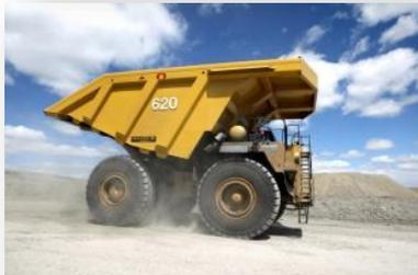
The **Westtech Flow Control Body**<sup>®</sup> has a revolutionary floor design that controls the flow of material out of the body during dumping. This more even flow greatly reduces dust generated when dumping, along with reducing wear on the body.
