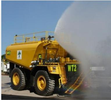
The JEC tank design has been in operation for over 20 years and the design principle is to compartment the tank to minimise the surge effect of the water with a series of baffles and allows for a lighter water tank. This translates into additional payload and less operating cost.
