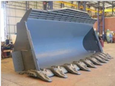
Austin Engineering design and manufacture **wheel loader buckets** from 1.5m<sup>3</sup> to 40m<sup>3</sup> with capacities to suit every OEM make and model. Available in a range of designs including large capacity lightweight, high lift, stemming, high dump, skeletal and grapple.
