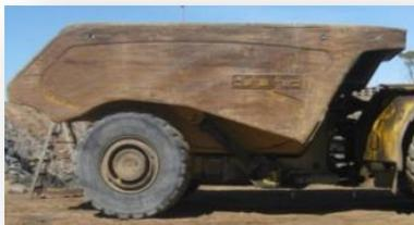
The **JEC underground mining tub** has been optimised with anti-carry back features and increased payload. Tub sizing is customised to suit site specific conditions, with the base tub design configured to be easily adaptable to a range of OEM trucks.
