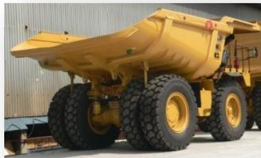
The key features of the design are the skeletal frame which complements the innovative replaceable floor. The replaceable floor eliminates the need for heavy, maintenance intensive wear liner plates. The floor can be easily removed and replaced in less time than replacing a full liner package.
