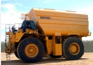
Austin Engineering's unique Westtech Stairway Access Tank module, unlike traditional water tank modules, has larger baffle openings with a direct line of travel to improve safety when performing confined space maintenance work.
