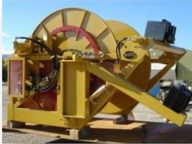
Westech cable handlers can be mounted on any chassis, allowing your operator to quickly and safely pick up or lay down cable at your mine site.
