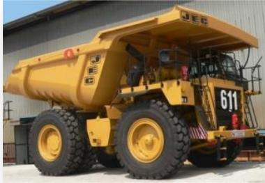
The **JEC body** design is a lighter weight modular design with the aim to improving payload, reducing material hang-up and reducing overall operating costs.
