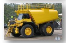
The JEC tank design has been in operation for over 20 years and the design principle is to compartment the tank to minimise the surge effect of the water with a series of baffles and allows for a lighter water tank. This translates into additional payload and less operating cost.
