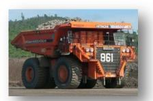
**Westech bodies** offer increased efficiency and lower operating costs due to their longevity and ability to maximise fleet capabilities. Three distinct body types are available – rock, coal, coal/overburden combo.
