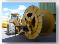
**Shovel Live Cable Handlers** are attached to and pulled behind the shovel, sled fashion, on pontoon runners protected by abrasion resistant liner plates.
